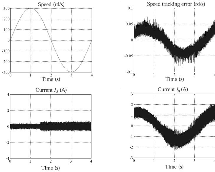
Figure 5. Speed tracking, with parameter variations at  $t = 1.5s$ , of PMSM
