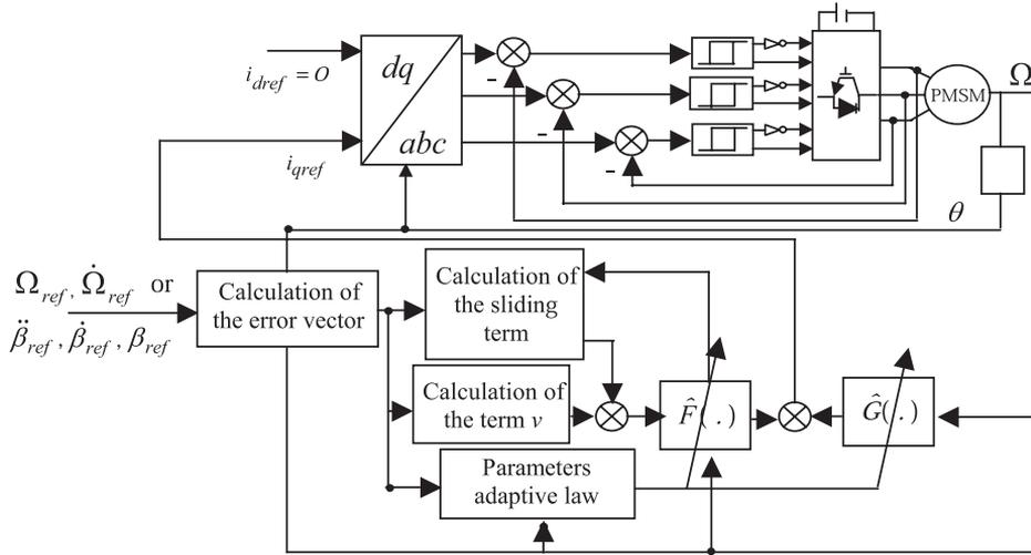
Figure 2. Direct adaptive fuzzy control scheme of permanent magnet motor
