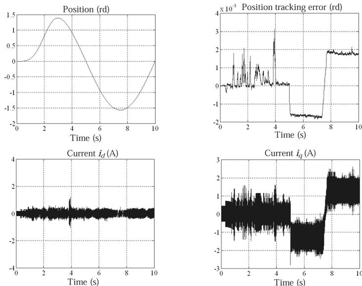
Figure 4. Position tracking, with the nominal load torque is applied at  $t = 5s$ , of PMSM
