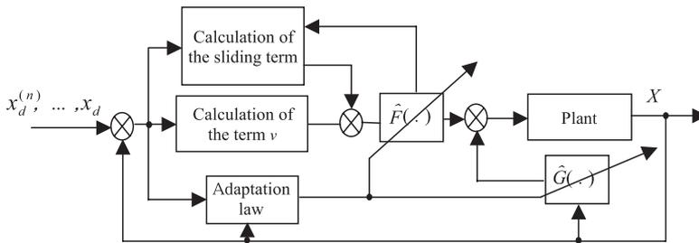
Figure 1. Structure of the direct fuzzy adaptive control
