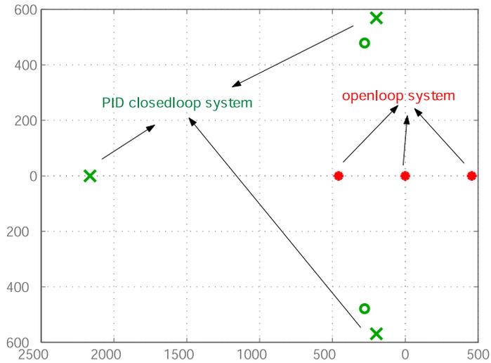
Figure 9. Pole-maps of the closed-loop and the open-loop systems
