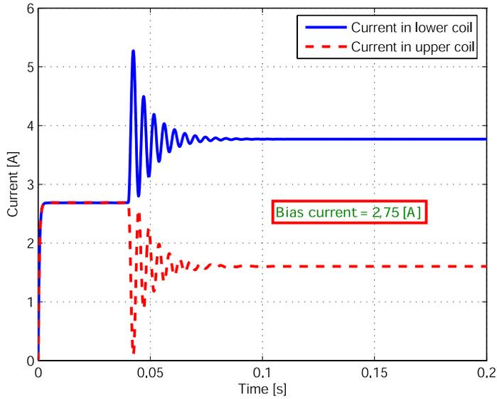
Figure 8. Current control signals in upper and lower coils of the magnetic bearings for step disturbance force  $F = 800\text{N}$
