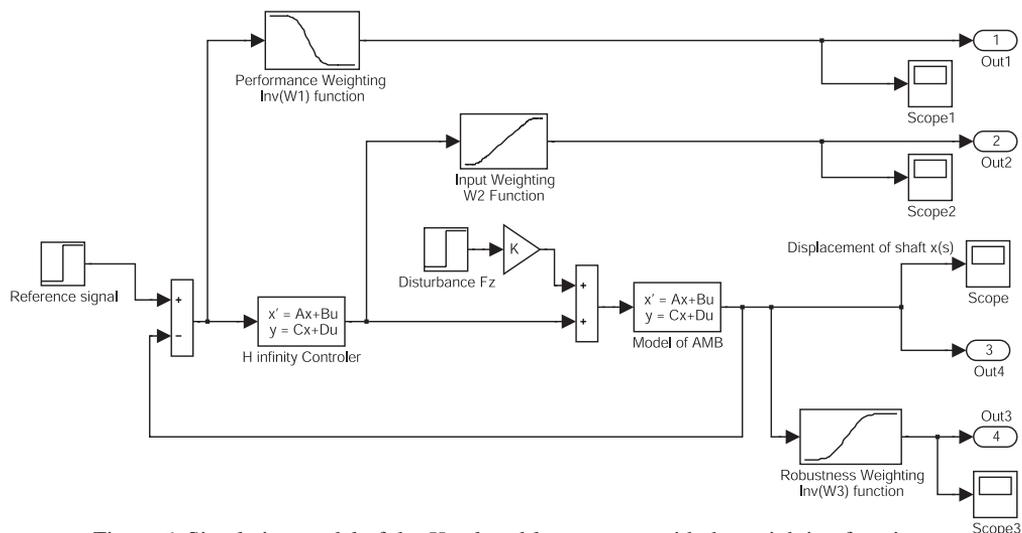
Figure 6. Simulation model of the  $H_\infty$  closed-loop system with the weighting functions
