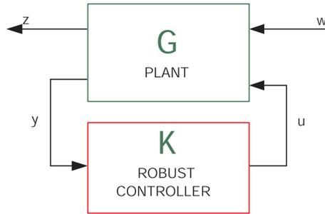
Figure 11. Diagram of the robust closed-loop system:  $w$ –reference signal,  $u$ –control signal,  $z$ –output signal,  $y$ –measurement signal
