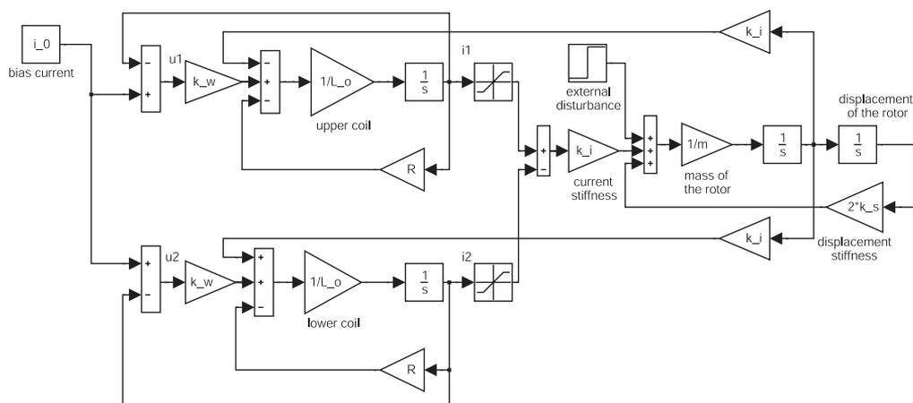
Figure 1. The nominal model of active magnetic suspension
