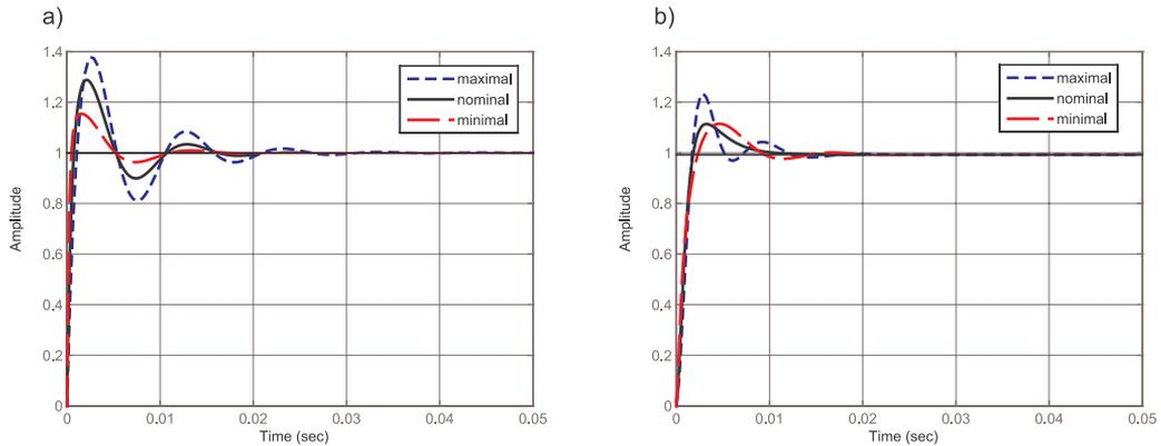
Figure 13. Step responses: a) PID closed-loop system, b)  $H_\infty$  closed-loop system
