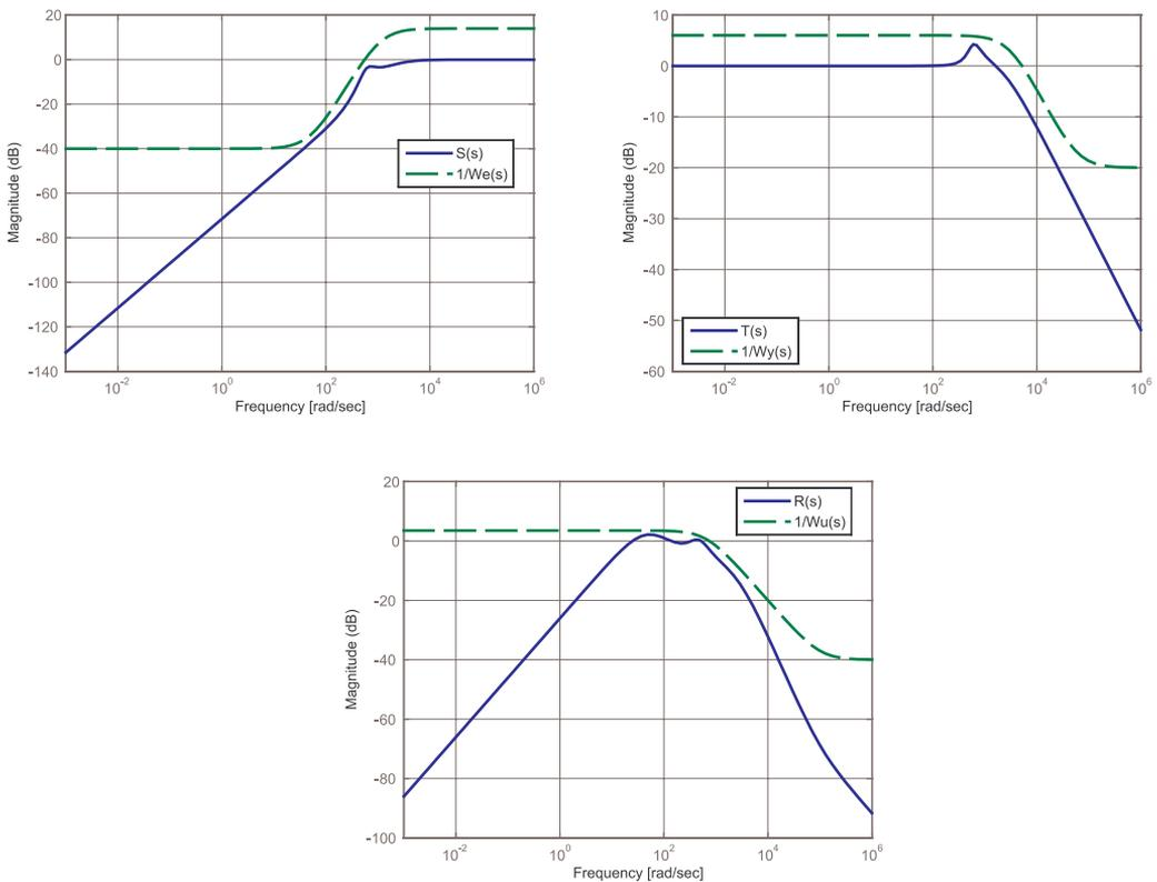
Figure 5. Amplitude-frequency plots of the weighting functions:  $W_u(s)$ ,  $W_e(s)$  and  $W_y(s)$
