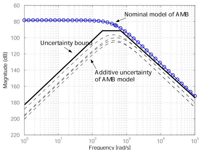
Figure 3. Amplitude-frequency plots of the plant nominal model, additive uncertainty  $\Delta_a(j\omega)$  and boundary function  $I_a(j\omega)$
