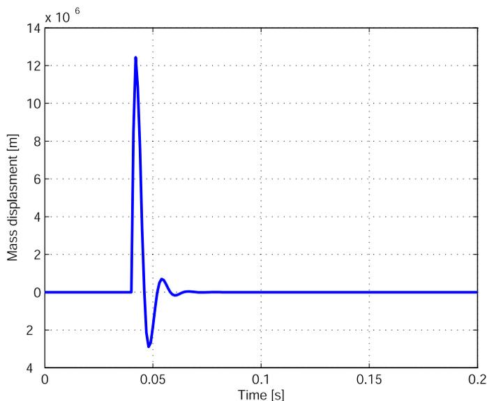
Figure 10. Step response of the PID closed-loop system for input force  $F = 600\text{N}$
