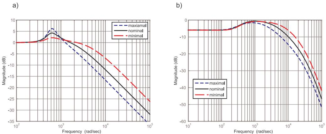
Figure 12. Frequency responses: a) PID closed-loop system, b)  $H_\infty$  closed-loop system
