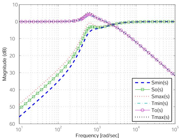
Figure 7. Amplitude-frequency plots of the functions:  $S(s)$  and  $T(s)$
