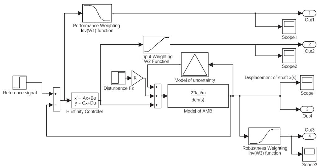
Figure 4. Simulation model of the  $H_\infty$  closed-loop system with the additive uncertainty
