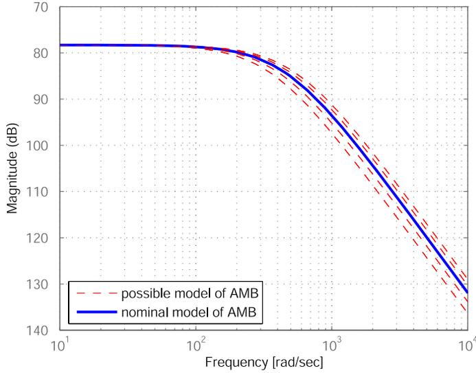
Figure 2. Amplitude-frequency characteristics of the nominal plant and for the plant with uncertain parameters  $k_i$  and  $k_s$
