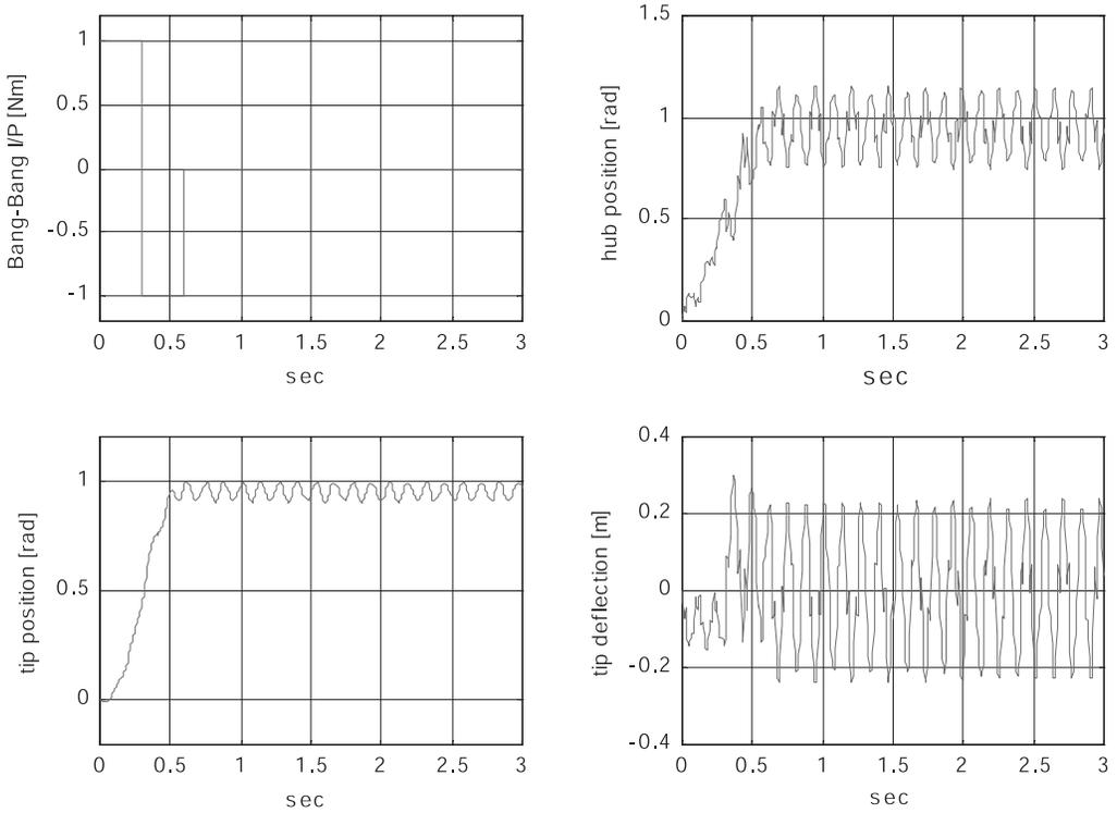
Figure 3. Bang-Bang input torque, hub, and tip displacement and tip deflection of the manipulator with payload  $m_p/m = 0.05$
