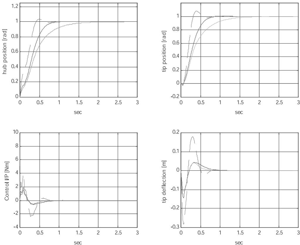
Figure 5. Step response of the flexible manipulator using SDRE controller with varying weighting
