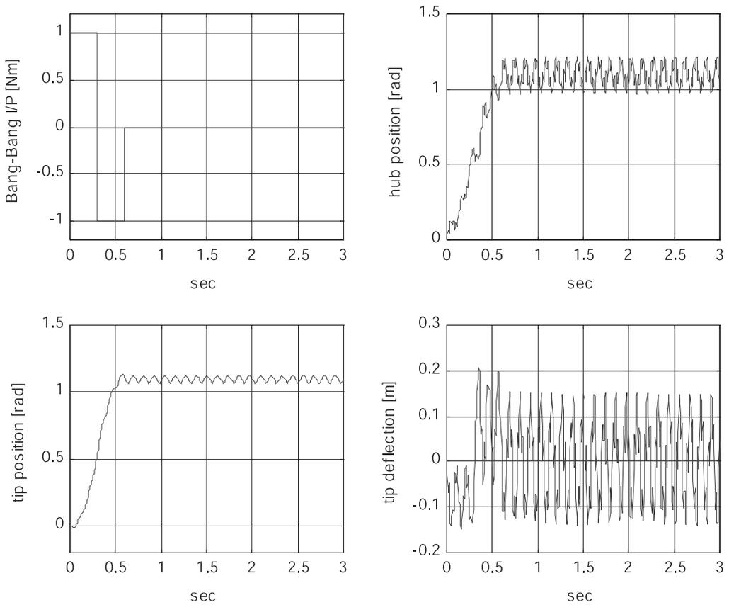
Figure 2. Bang-Bang input torque, hub and tip displacement, and tip deflection of the manipulator without payload
