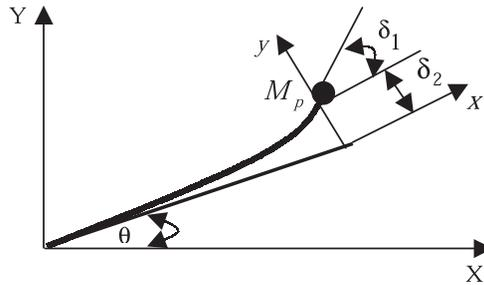
Figure 1. Geometric and Generalized Coordinates of a flexible link
