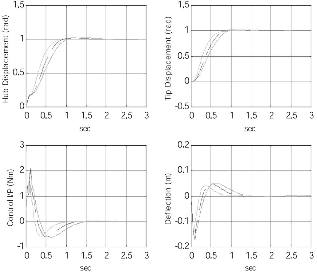
Figure 6. Step response of the flexible manipulator using SDRE controller with  $m_p/m = 0, 0.25, 0.5$  payload
