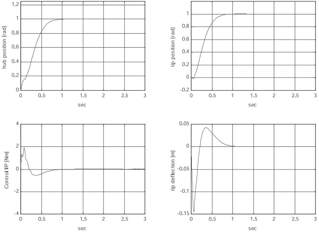
Figure 4. Step response of the flexible manipulator using SDRE controller without payload
