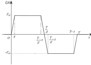
Figure 5. Trapezoidal control function
