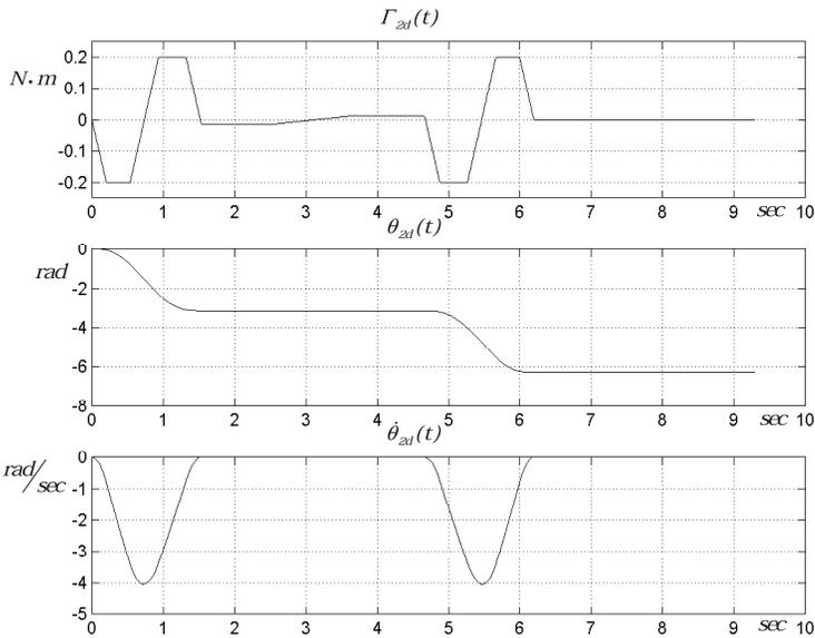
Figure 16. Feed-forward torque and reference trajectory for the second link of two-link arm
