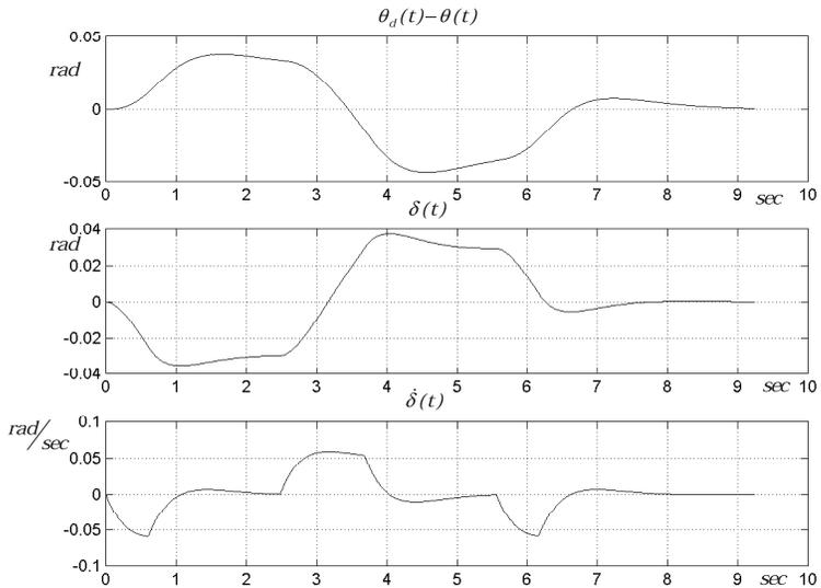
Figure 8. The error tracking of the angle, the elastic variable and its time derivative for one-link arm under control (21)
