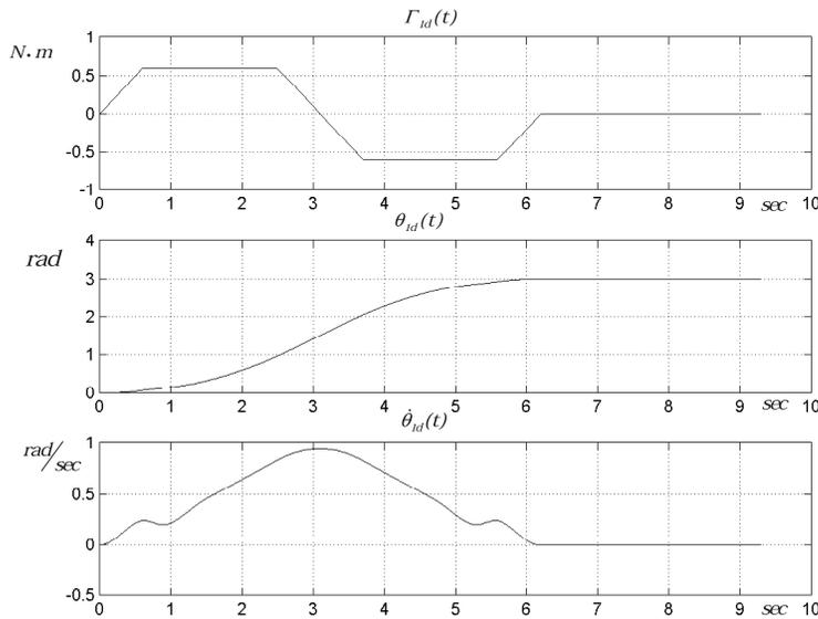
Figure 13. Feed-forward torque and reference trajectory for the first link of two-link arm with flexible joints
