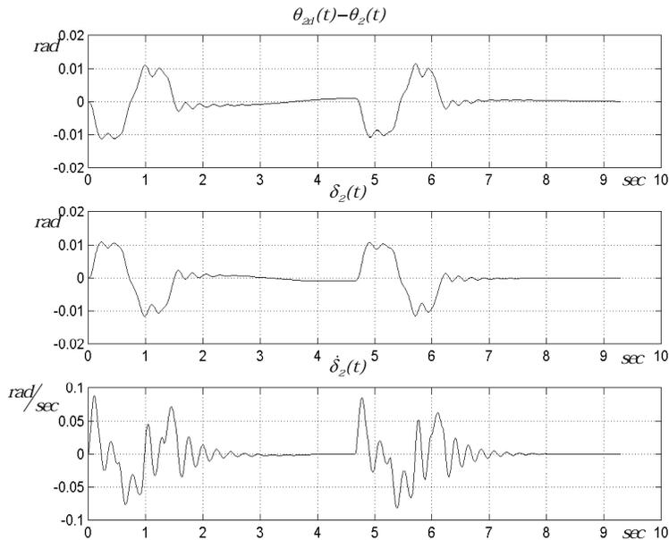
Figure 18. The error tracking of the angle, the elastic variable and its time derivative for the second link of two-link arm under control (43)
