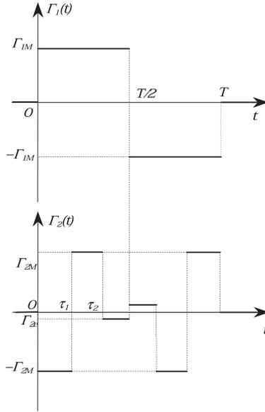
Figure 10. Discontinuous quasi-time-optimal control functions
