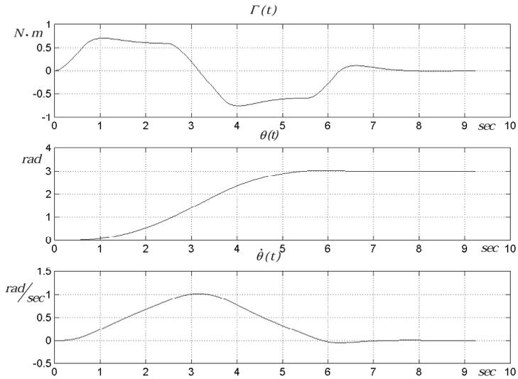
Figure 7. The control torque, angle and angular velocity for one-link arm under control (21)
