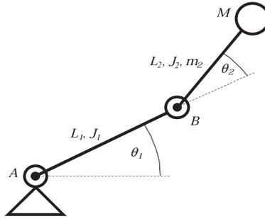
Figure 9. Scheme of an arm with two links
