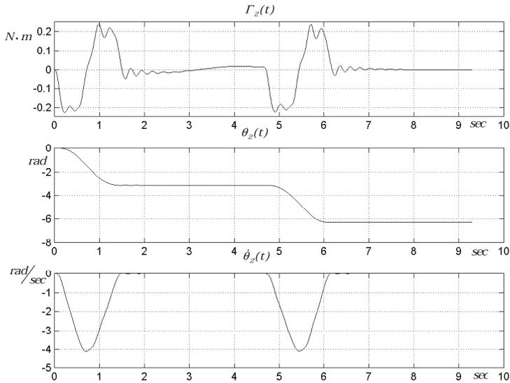
Figure 17. The control torque, angle and angular velocity for the second link of two-link arm under control (43)
