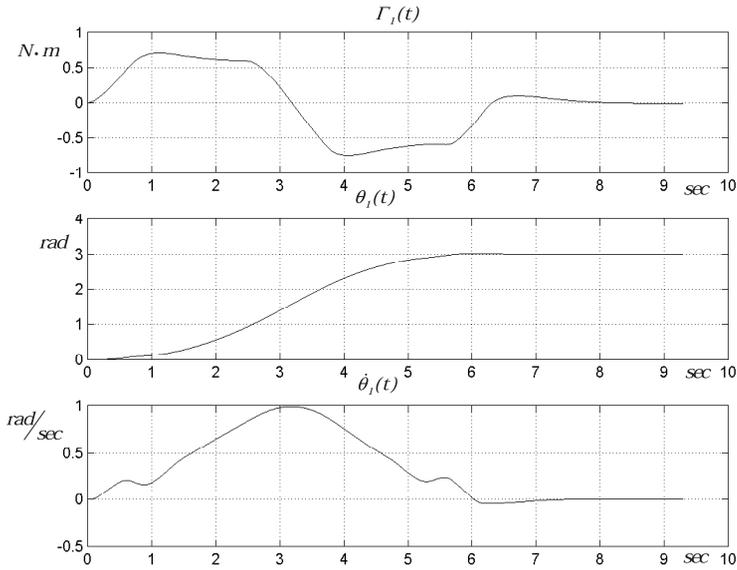
Figure 14. The control torque, angle and angular velocity for the first link of two-link arm under control (43)
