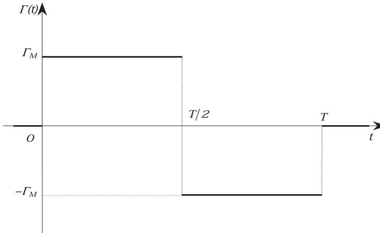
Figure 2. Time-optimal control for the system (9)
