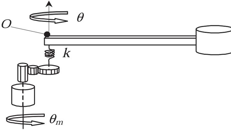
Figure 1. Scheme of the link with flexible joint
