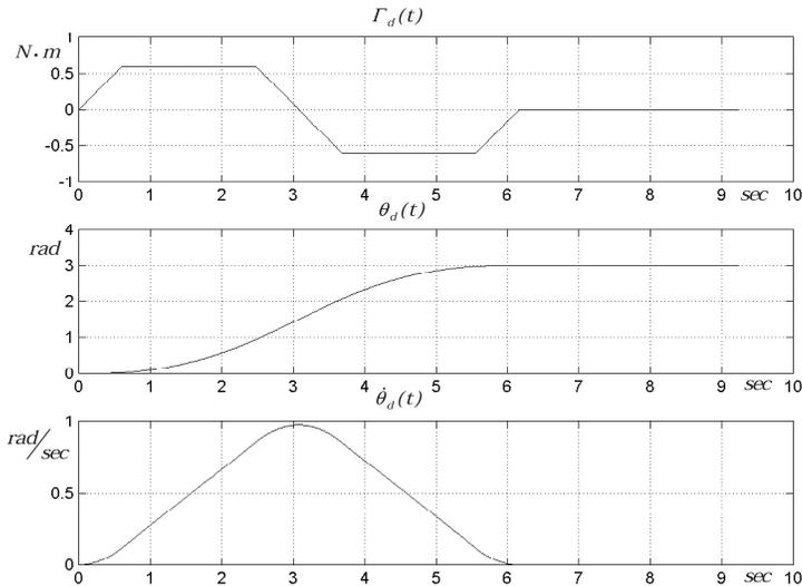
Figure 6. Feed-forward torque and reference trajectory for one-link arm with flexible joint
