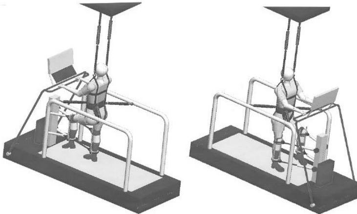
Figure 14. Full BWST arrangement with PSD in two oblique views
