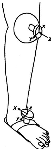
Figure 2. Placement of F/T sensors
