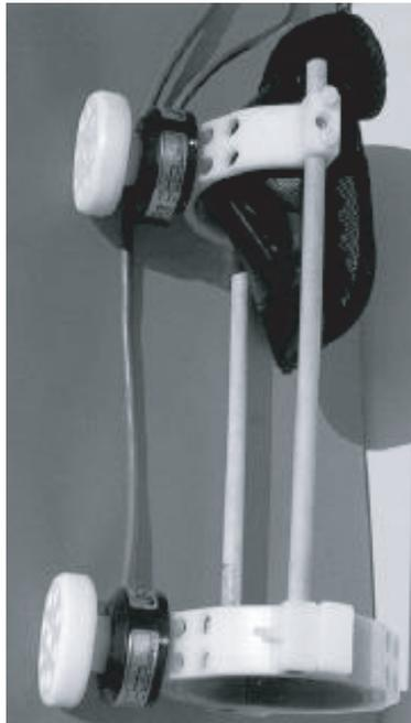
Figure 8. Leg exoskeleton frame equipped with two F/T&A sensors units. A kneecap is part of the frame.
