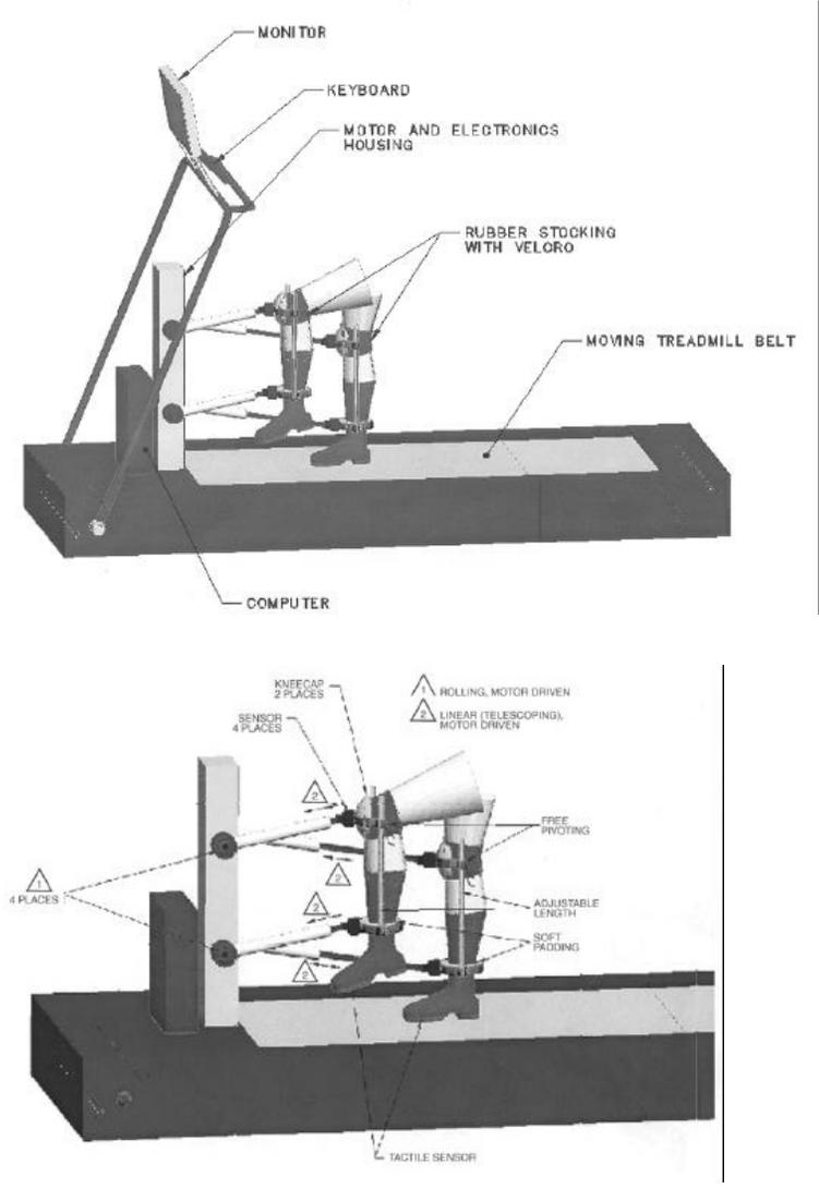
Figure 11. A possible PSD system architecture uses two two-degree-of-freedom robot arms acting in the sagittal plane and connected to an exoskeleton leg
