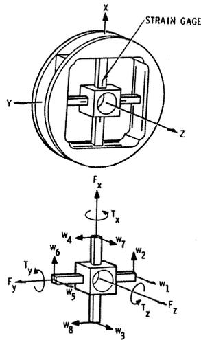
Figure 4. F/T sensors mechanical frame with output in cartesian frame
