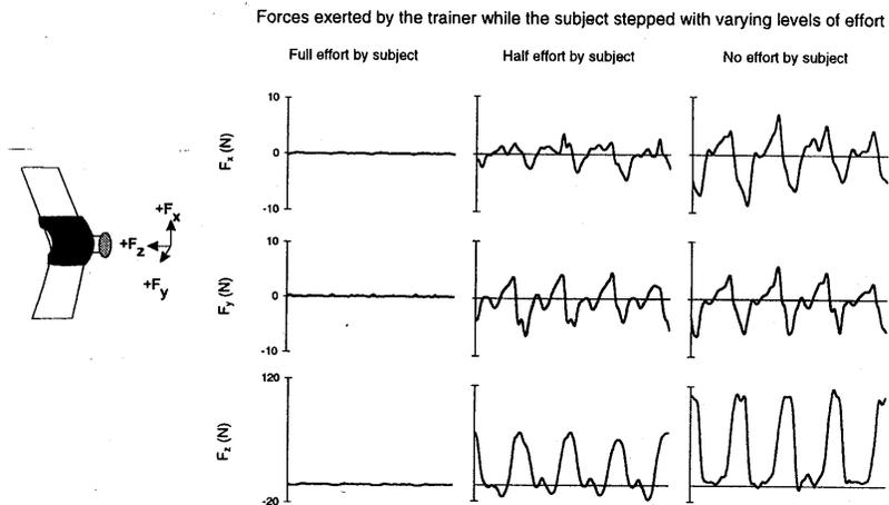
Figure 5. F/T sensors functionality test at knee
