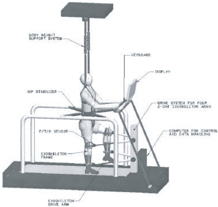
Figure 13. Full BWST arrangement with PSD, with major system elements indicated
