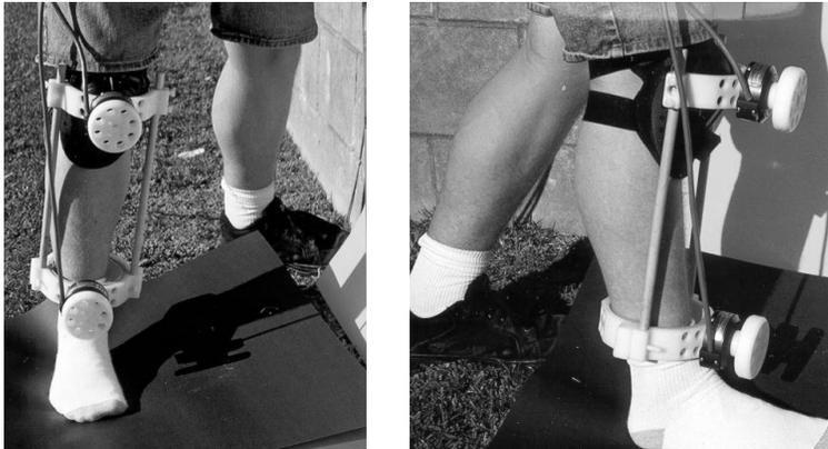
Figure 10. Sensor-equipped exoskeleton attached to a leg for fitting tests and adjustments. The lower ring to be patted against the leg.
