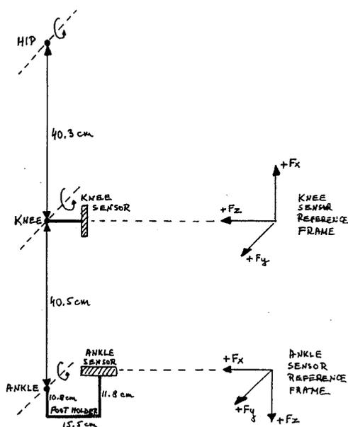
Figure 6. An application case geometry
