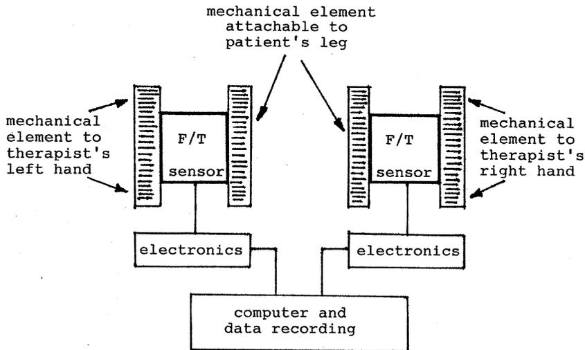
Figure 1. Two-hand force torque (F/T) measurement system
